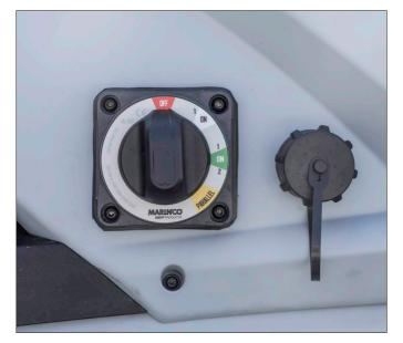
Auxilliary electrical system With two parallell separated circuits which provides optimized electric redundancy. If one circuit breaks you just switch to circuit 2.
