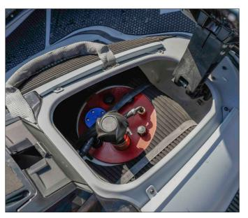
**Extended fuel capacity** 70 + 30 Litre fuel capacity divided on 2 separate tanks, providing an effective range of 100-120 nautical miles.
