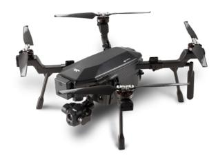
SIRAS is an affordable, easy-to-fly, IP54-rated professional drone with an interchangeable payload system for industrial and utilities inspection, firefighting, law enforcement, and search and rescue missions. With front collision avoidance, hot swappable batteries, a 31-minute flight time, and no restrictive geofencing, professional UAV pilots can fly safely when and where the mission demands.
